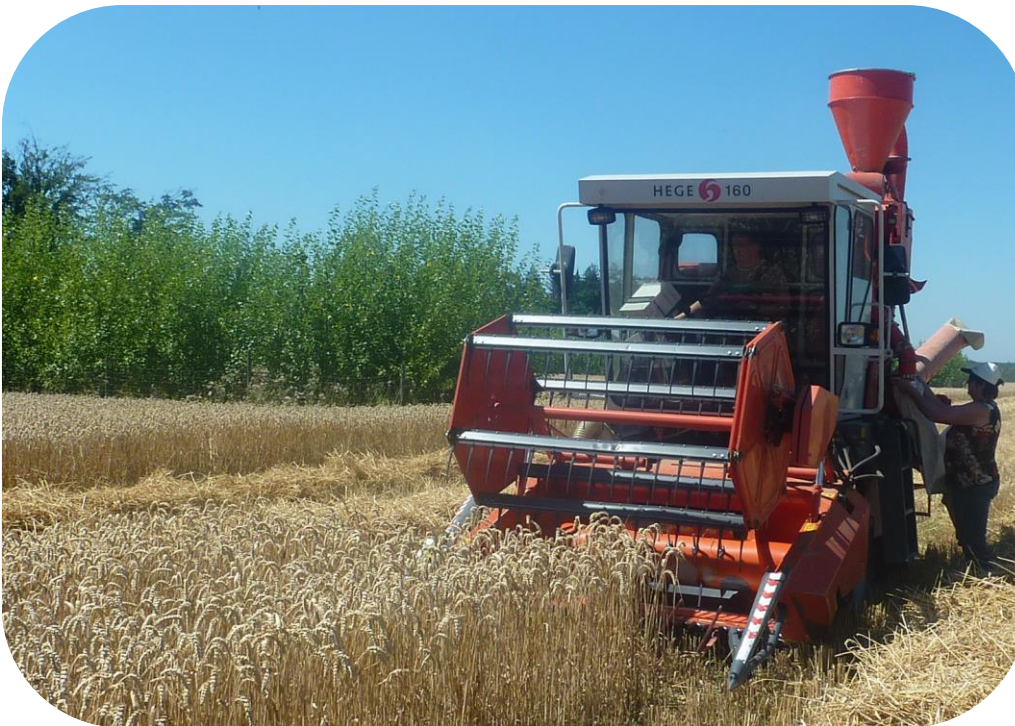
Yield measurements using a plot combine
